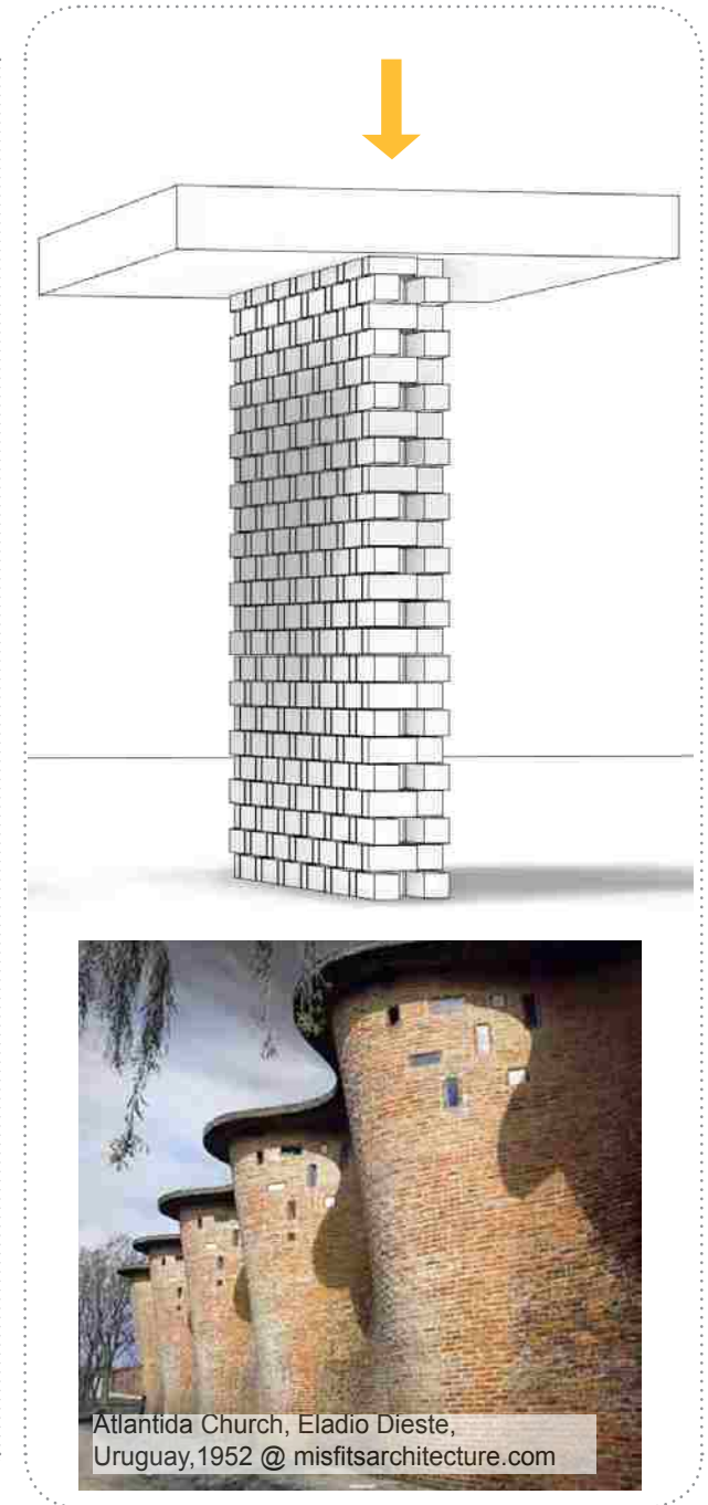
Figure 20: Multiple-wythe brick wall
